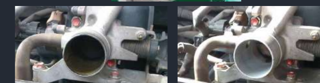
BEFORE (Throttle body condition after 60,000 km)
