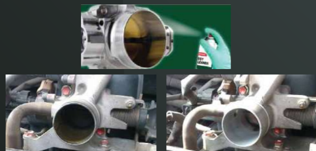
BEFORE (Throttle body condition after 60,000 km)
